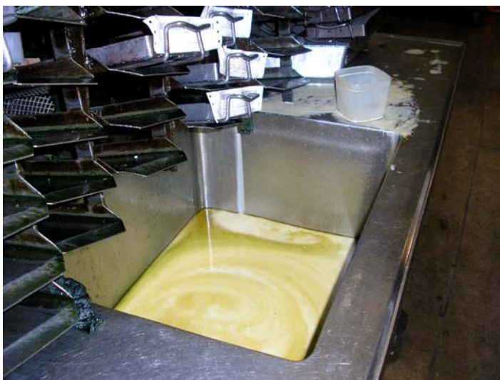
Figure 2-22. Rust Inhibitor Tank at Deltronic
