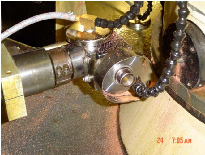
Figure 2-10 Cutting Machine with Near Dry Lubrication at Weldcraft
