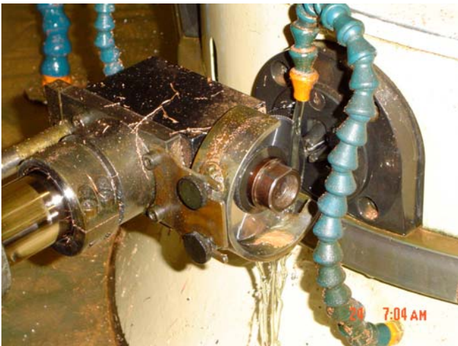
Figure 2-9. Flooding Lubrication at Weldcraft
