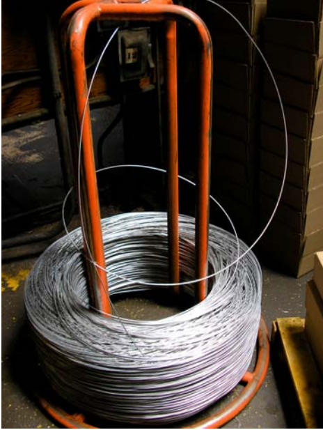
Figure 2-16. Feed Wire Coil at Winders & LeBlanc
